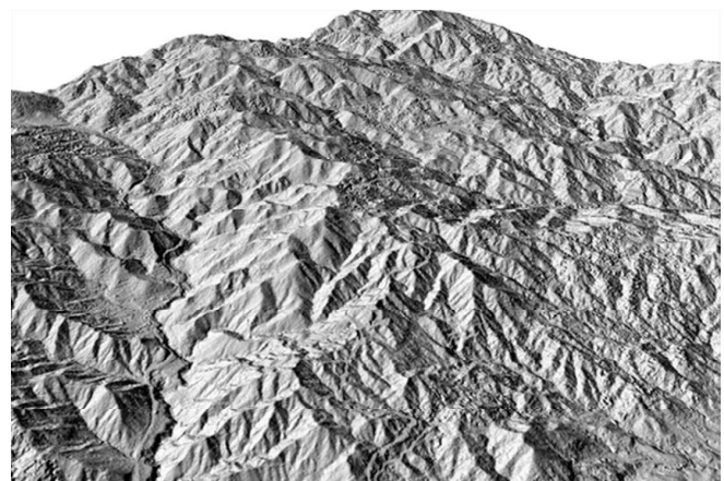
Fig. 6. Post-fire DSM generated from the images acquired in July 2014
