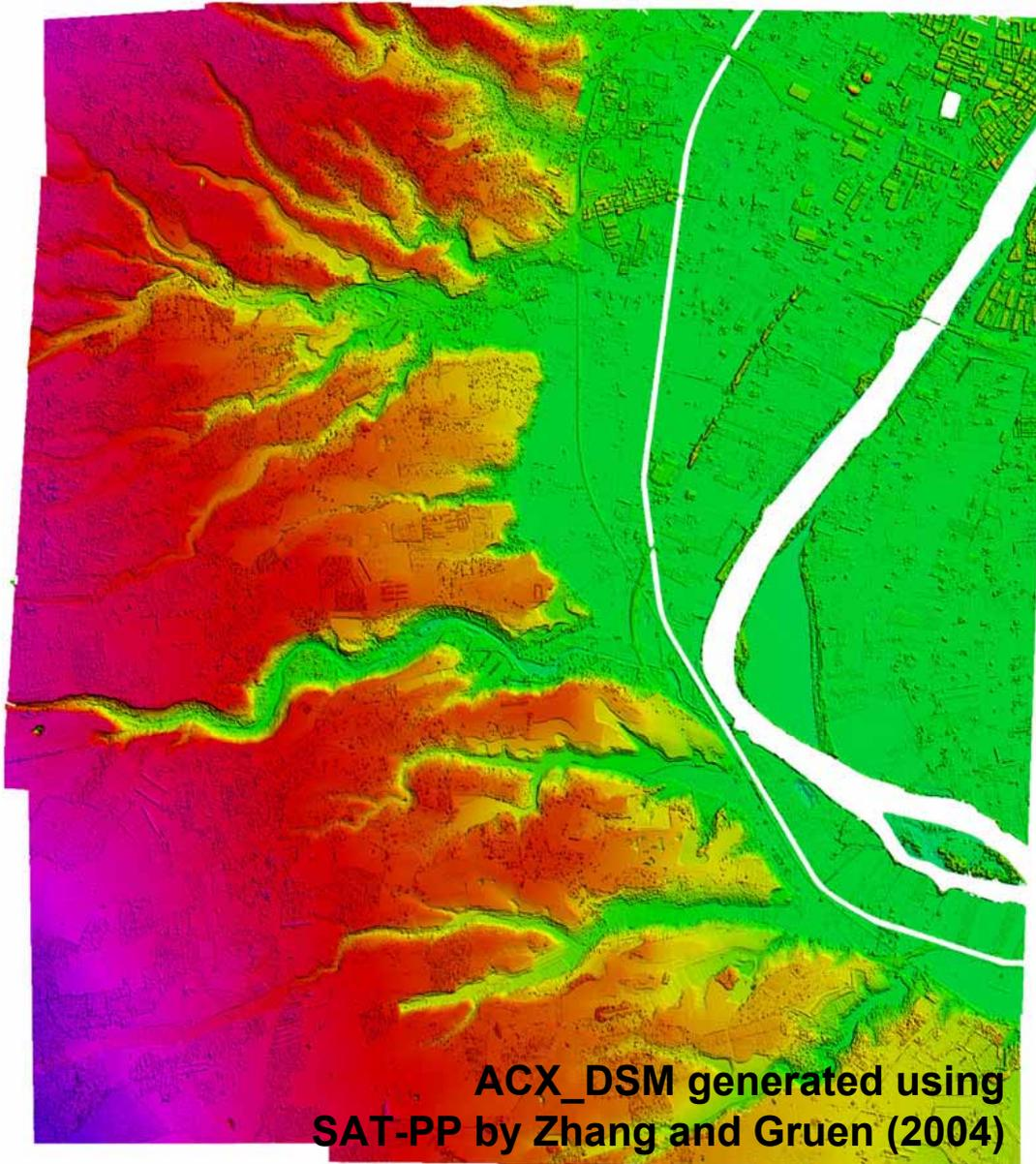
**Task:** Quality evaluation of the DSMs derived by **DMC digital airborne camera** imagery
