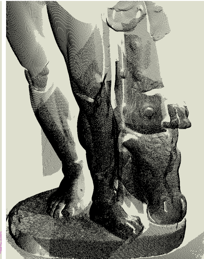
Example: Registration of first 10 scans Note: 3x3 down-sampling for better visualization
