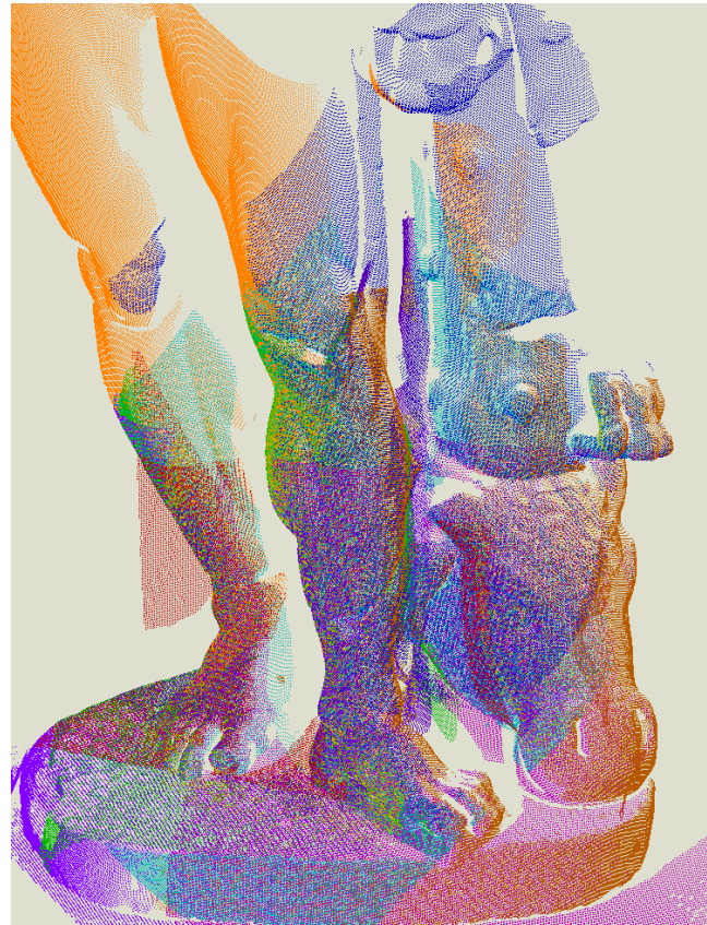
Example: Registration of first 10 scans Note: 3x3 down-sampling for better visualization
