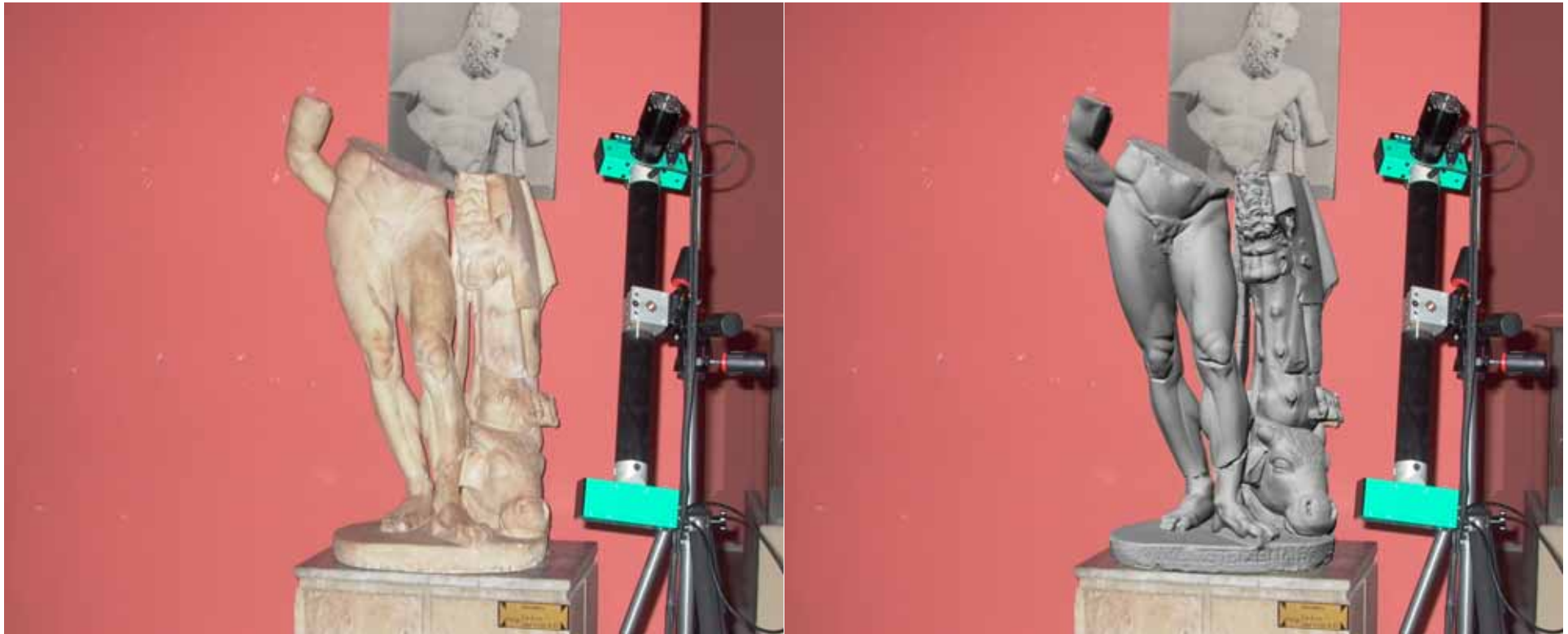
Back projection of the 3D model into image space
