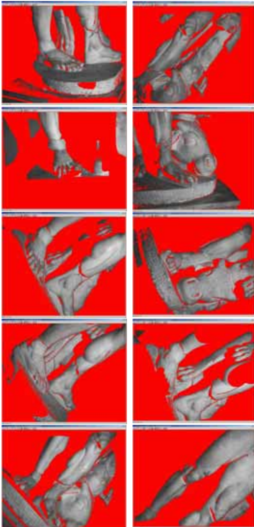
Example: Registration of first 10 scans Note: 3x3 down-sampling for better visualization
