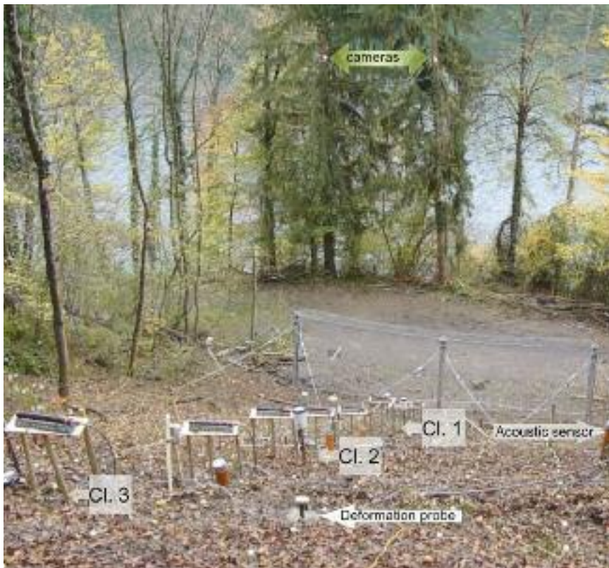
Fig. 4: Location of the instrumentation clusters (Cl. 1 – 3), the sprinklers and the photogrammetry cameras.
