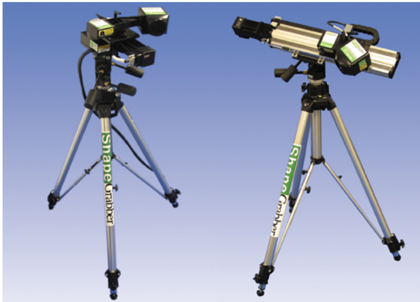
ShapeGrabber – BIRIS Small object volume High accuracy ~ 50-100micron
