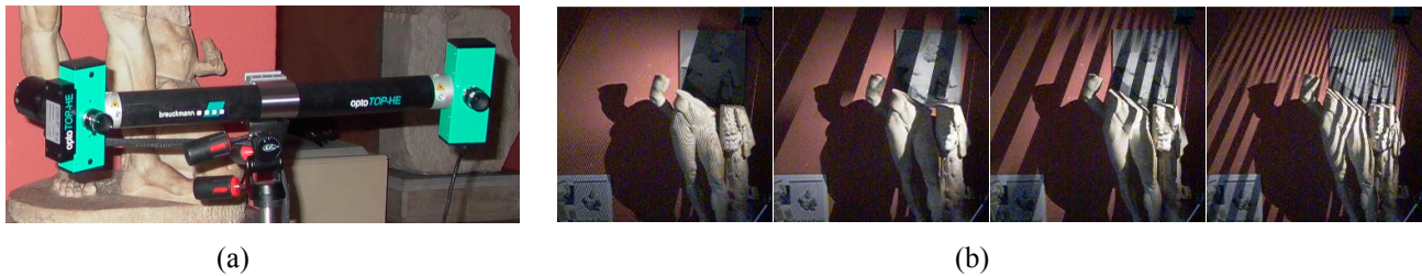
Fig.3. (a) The optoTOP-HE sensor, (b) first 4 fringe projections of a scan of the optoTOP-HE sensor.
