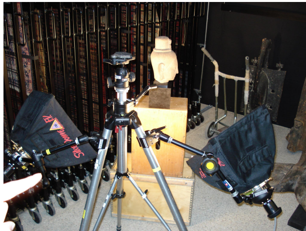
Fig.9. Illumination system used for the texture mapping in Museum Rietberg.
