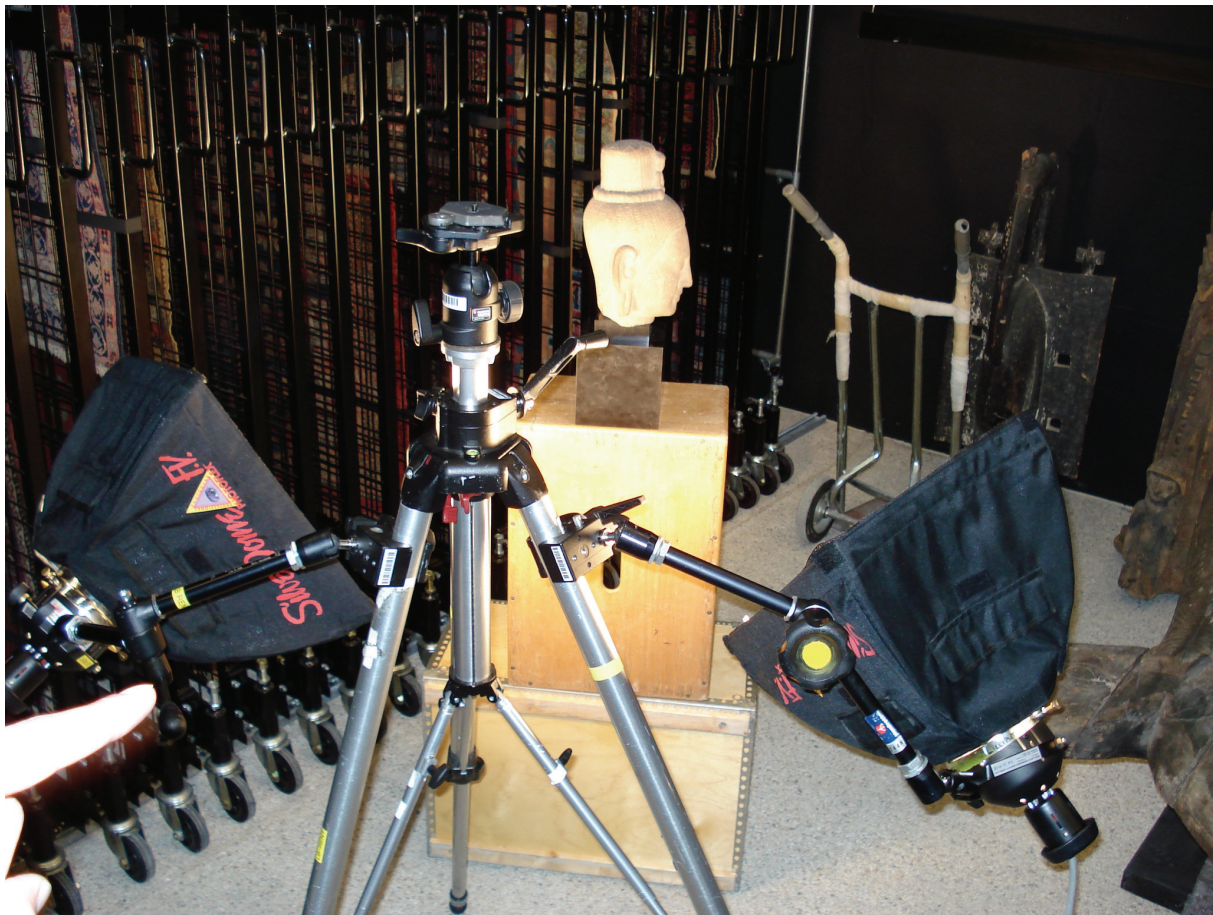
Figure 20. The illumination system used for the texture mapping.
