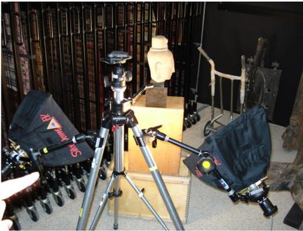
Figure 6. Illumination system used for the texture mapping
