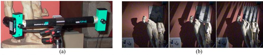
Figure 3. (a) The optoTOP-HE sensor, (b) and its first 3 fringe projections.
