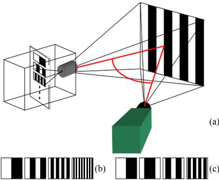
Figure 2. (a) Setup of a fringe projection system with the natural binary codification, (b) natural binary code, (c) Gray binary code.
