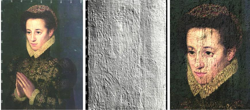
Figure 7. Recorded 3D model with color (left), 3D data after background compensation (middle), face, Z co-ordinate magnified by a factor of 50 (right).
