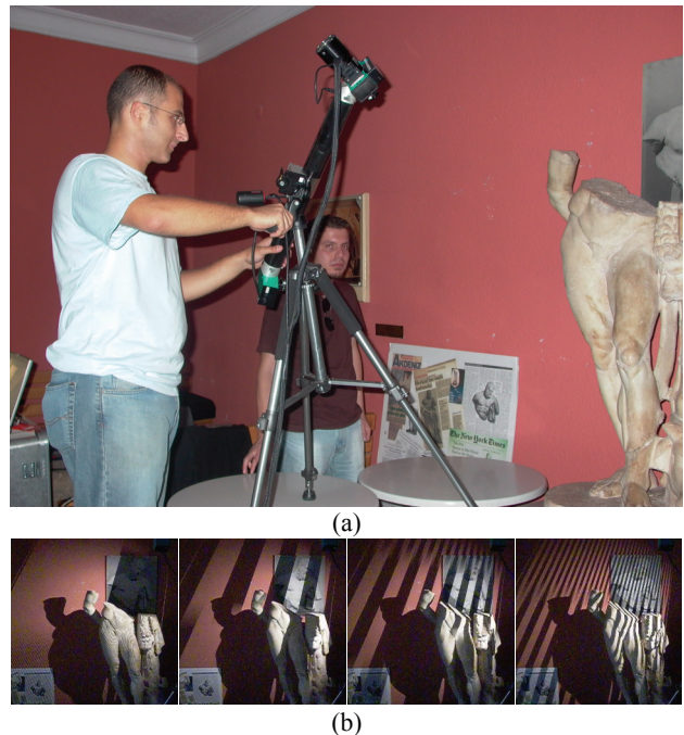
Figure 5. (a) Preparation, (b) first 4 fringe projections of a scan
