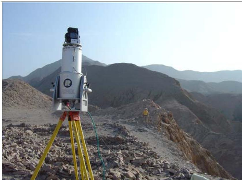
Figure 3. The Riegl LMS-Z420i scanner is at the site.
